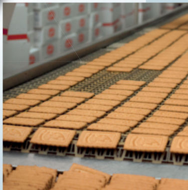
Conveyor belt in the spray zone
