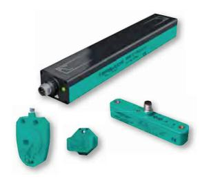
The Inductive Position Coding System PCI consists of the PCI head and multiple actuators, which encode the position by the particular arrangement to each other. The PCI system is particularly suitable for precise angle determination of slewing bearings in heavy machinery.
