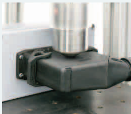
Impact of falling hammer weighing 1.7 kg
