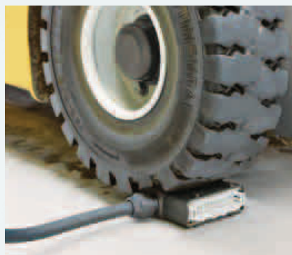
Extreme load due to roll-over with a forklift truck
