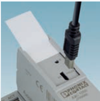
The USB connection provides fast access, e.g., for diagnostics
