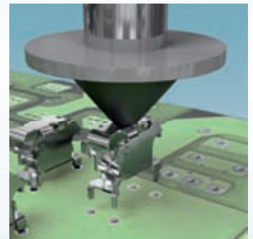
Optimized for SMT and THR mounting – due to integrated suction areas.
