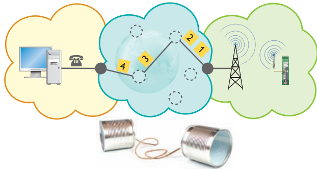
Fig. 11 ► Put very simply, data transmission via CSD is comparable to an "exclusive cable" for customers.
