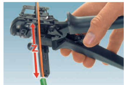
Tool for on-site assembly.
