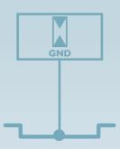
**Direct grounding** In the PT-IQ-...-UT protection modules, the connection terminal blocks for the shield or the reference potential are directly connected to the DIN rail via the metal mounting foot.
