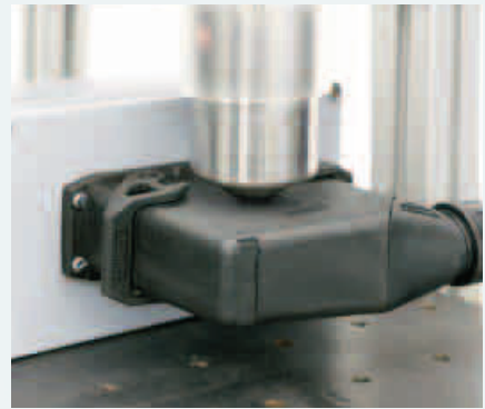
Impact of falling hammer weighing 1.7 kg
