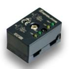
The terminator reduces reflections at the cable ends and improves communication. With the integrated multiple impedance and two options for inserting the flat cable, a network length of 200 m has been achieved with all tested topologies and cable loads. The device also displays the voltage drop for both AS-Interface and AUX. The one-piece terminator can be fitted to the flat cable without additional accessories.
